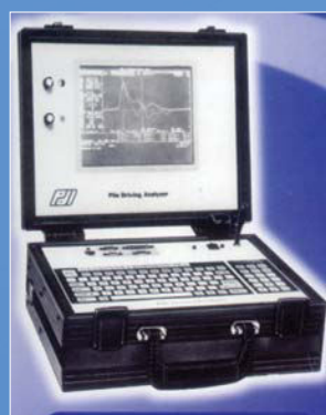
Dynamic Pile Testing-PDA System
